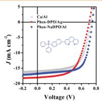
The organic molecule Phen-NaDPO that possesses characteristics of a facile synthesis/purification, a high  $T_g$ , and attactive electron transport, is successfully shown as an promising cathode interlayer to improve the PCE. Consequently, a PCE of 7.5% and 8.56% is reported respectively for Phen-NaDPO/Ag and Phen-Na-DPO/Al devices utilizing PTB7:PC71BM active layer, which compares well with that of the Ca/Al device.
