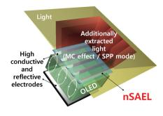
An invisible nanosized stripe auxiliary electrode layer (nSAEL) for OLEDs that can avoid the shortcomings of conventional microsized layers while maintaining high optical uniformity due to the improved conductivity of the electrode is proposed. An additional advantage is that the structure of the nSAEL increases light extraction by utilizing the microcavity (MC) effect and the outcoupled surface plasmon polariton (SPP) mode.
