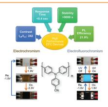
A high-performance electrofluorochromic (EFC) device of poly(4-cyanotriphenylamine) (CN-PTPA) as active layer is readily fabricated and exhibits high photoluminescent (PL) quantum yield of 21.9% in film state, high PL contrast ratio  $(I_{\rm off}/I_{\rm on})$  of 242 from a fluorescent neutral state to a non-fluorescent oxidized state, rapid response time less than 0.4 s. and excellent EFC stability longer than 9000 s.
