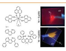
New Eu(III) and Gd(III) complexes combine efficient excitation with blue light, strong emission, and efficient oxygen quenching capabilities. They are used in advanced oxygen sensing materials including planar optodes and nanosensors.
