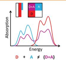
Charge separation at the donor-acceptor interface in organic solar cells may be assisted by interfacial charge transfer type complexes that prevail already in the ground state. In bilayer solar cells, a reduced absorption that correlates with solar cell efficiency is observed and attributed to the formation of interfacial ground state charge transfer complexes.
