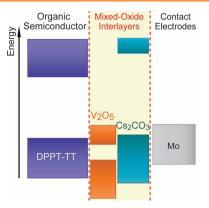
A gradual control of the metal electrode's work function ( $\Phi$ ) by incorporating solution-processed mixed contact interlayer of transition metal salts (Cs2CO3 and  $V_2O_5$ ). Low-cost Mo electrode with  $\Phi =$ 4.5 eV is finely modulated between 4.2 eV and 4.8 eV by controlling mixed concentration, which are used as common source/drain electrodes in high-mobility ambipolar polymer semiconductor OFETs and complementary-like inverter circuit.
